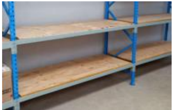
Decking between braces horizontal closed wood
